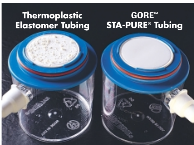
Spallation debris collected onto a microporous filter membrane after recirculating water for 48 hours through thermoplastic elastomer tubing (left) and GORE™ STA-PURE® tubing (right). The thermoplastic elastomer tube produces particles of rubber, inorganic filler, and plasticizer.
